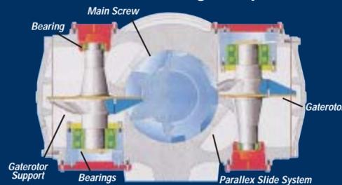
The standard Vilter Single Screw Compressor (as shown in this end view drawing) consists of two rotating gaterotor assemblies and a main screw assembly. All bearings are pressure fed with oil.
