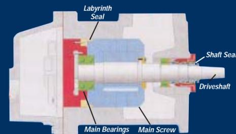
This side view cross-sectional drawing of a Vilter oil flooded Single Screw illustrates the suction and the discharge ports as well as the various seals and driveshaft.
